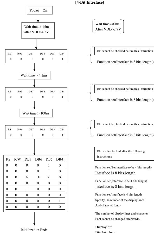
BF cannot be checked before this instruction Function set(Interface is 8 bits length.) BF cannot be checked before this instruction Function set(Interface is 8 bits length.) BF can be checked after the following instructions Function set(Set interface to be 4 bits length) Interface is 8 bits length. Function set(Interface to be 4 bits length) Interface is 8 bits length.
